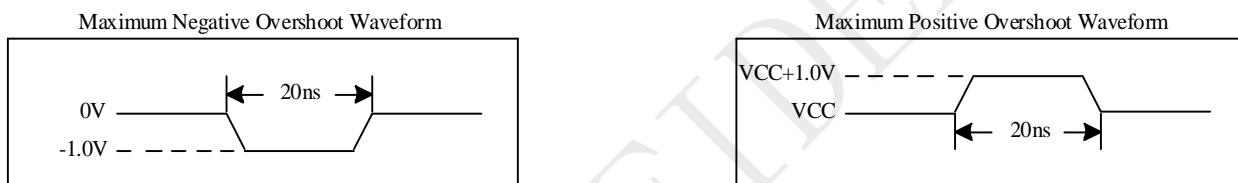
Figure 5-2 Input Test Waveforms and Measurement Level
